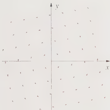
Figure 7.7 A pictorial representation of the vector field described by \mathbf{v} = -\omega y \mathbf{i} + \omega x \mathbf{j} .
