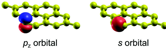
Figure 3.33 The Wannier functions of graphene includes p_z (left) and s (right) orbitals.
