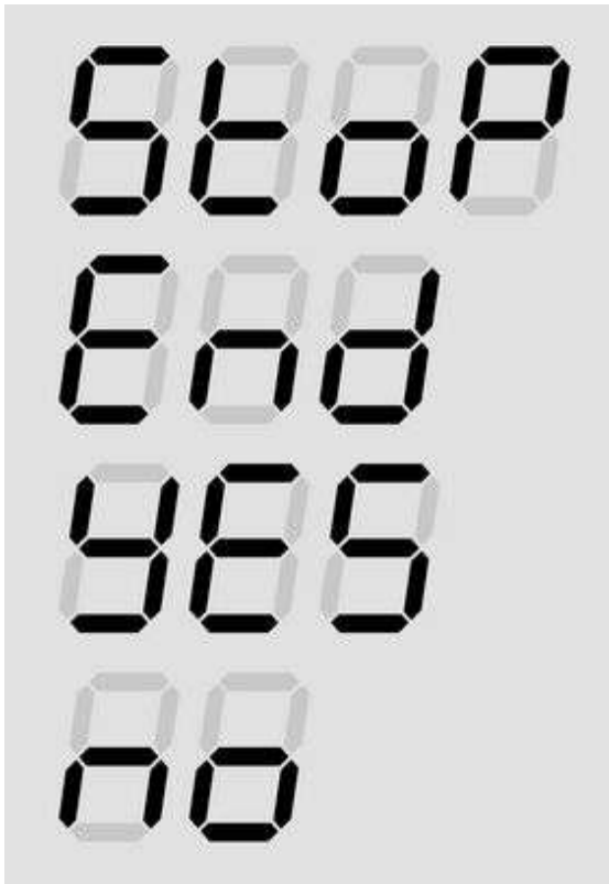
Figure 17-6. Basic text messages can be generated with 7-segment displays, although they cannot contain alphabetical letters that use diagonal strokes.
