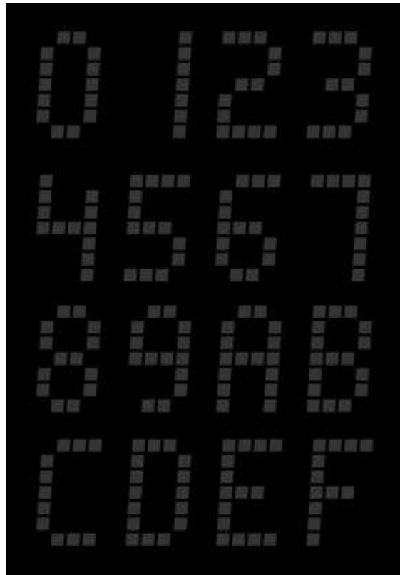
Figure 24-16. Sixteen possible outputs that can be displayed by the Texas Instruments TIL311 to show a hexadecimal value in response to a four-digit binary input.
