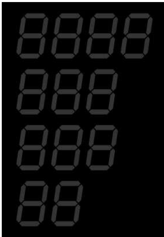
Figure 24-4. Basic text messages can be generated with seven-segment displays, although they cannot represent alphabetical letters containing diagonal strokes.
