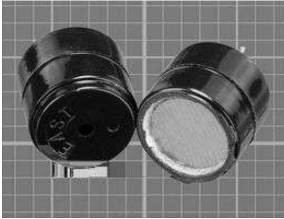
Figure 28-2. An audio indicator approximately 0.5" in diameter, partially disassembled on the right, revealing its brass diaphragm.
