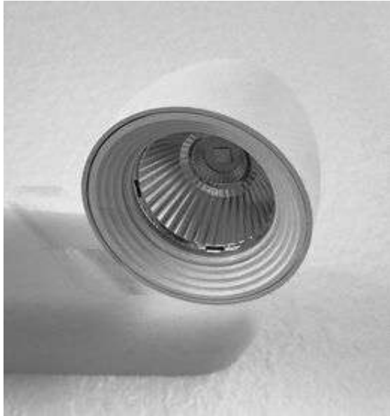
Figure 23-1. A small LED reflector-light emulating a halogen fixture. Note the square of yellow phosphors mounted on the diode.
