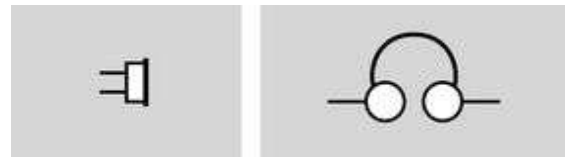
Figure 29-1. Schematic symbols for a single earphone or headphone (left) and a pair of headphones (right).
