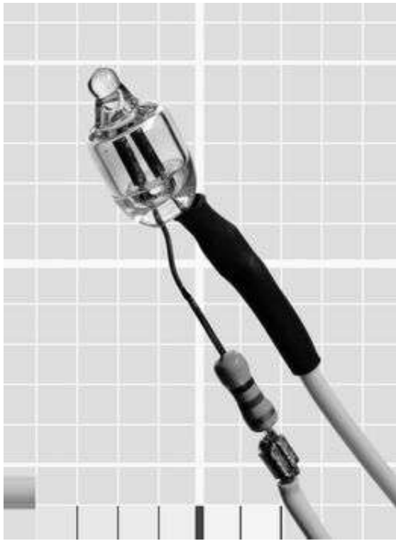
Figure 19-2. A typical neon bulb with series resistor attached to one lead.
