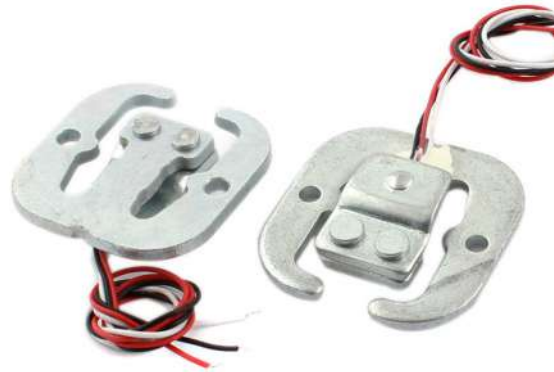
Figure 12-5 Two force sensors suitable for a bathroom scale, each containing a pair of strain gauges that will flex oppositely under load.
