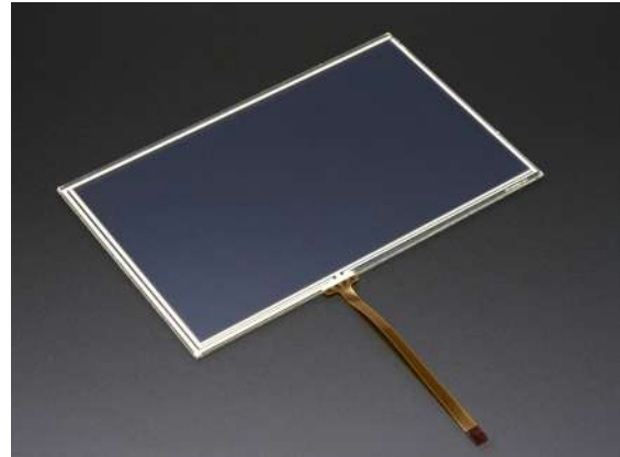
Figure 14-3 This resistive touch screen is intended for use as a layer applied to a 7-inch video display. The screen is available from Adafruit.
