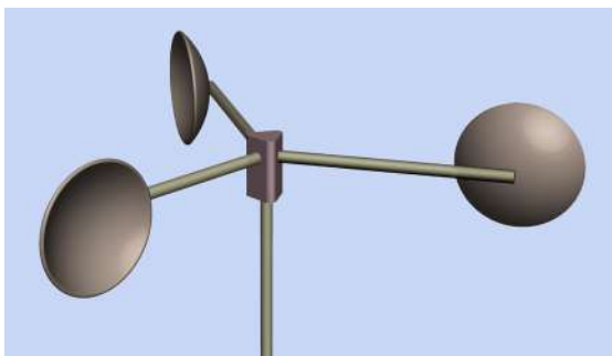
Figure 19-1 The basic design of a meteorological cup anemometer.
