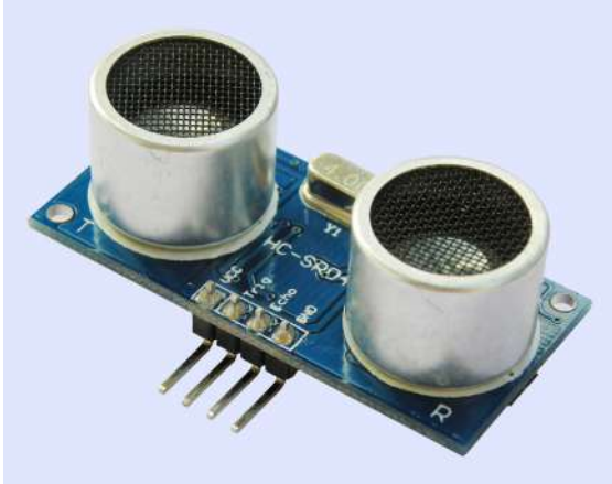
Figure 5-4 The HC-SR04 is a very low-cost import that can provide acceptable performance when used with an external microcontroller.
