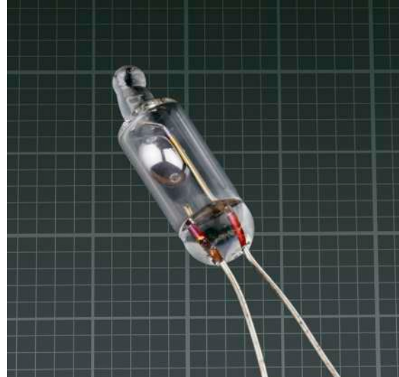
Figure 8-6 Small mercury switch rated for 0.3A at 24VDC or 24VAC. Larger mercury switches can switch more power; 1A at 230V is common. The background grid is in millimeters.
