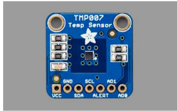
Figure 28-6 The TMP007 sensor mounted on a breakout board from Adafruit.
