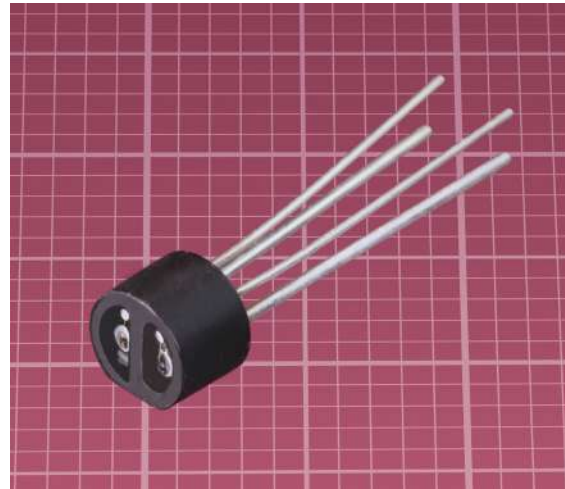
Figure 3-7 The Rodan RT-530 is a small object-presence sensor with a limited range typical of this type of retroreflective component. The background grid is in millimeters.
