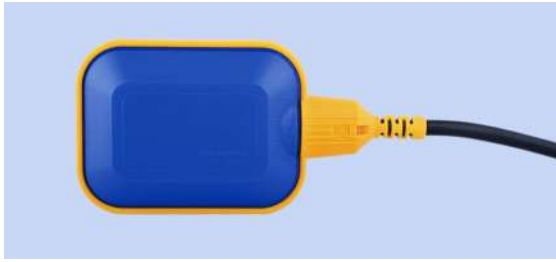
Figure 15-3 An air-filled float that switches external power depending on its orientation.
