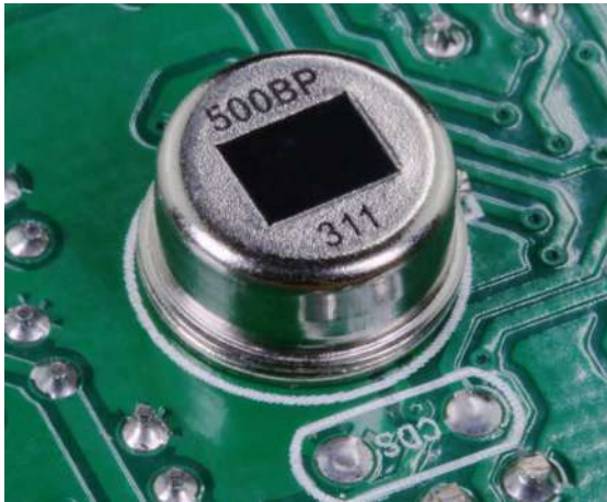
Figure 4-3 A pyroelectric detector mounted on a small circuit board in a passive infrared radiation sensor.
