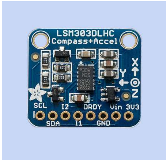
Figure 2-7 The LSM303 is a chip manufactured by STMicroelectronics. It is shown here on a breakout board from Adafruit.
