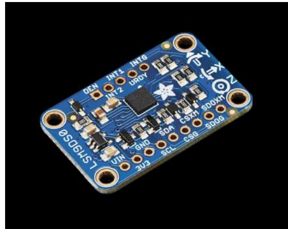
Figure 10-6 This breakout board from Adafruit is built around an LSM9DS0 chip that combines accelerometers with gyroscopes and magnetometers.
