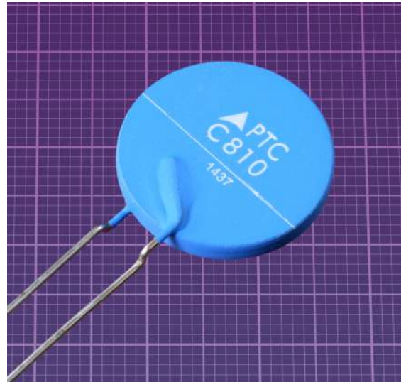
Figure 24-5 A large over-current protection PTC thermistor. The background grid is in millimeters.
