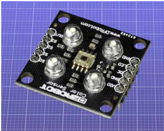
Figure 21-5 This breakout board from Robot Shop uses the Taos TCS3200 chip to analyze the color of incident light.
