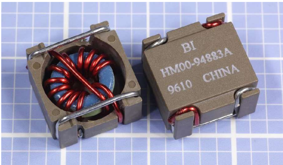
Figure 14-16. A larger-sized surface-mount toroidal inductor (viewed from the bottom, at left, and from the top, at right). It is rated at 3.8\mu\text{H} .
