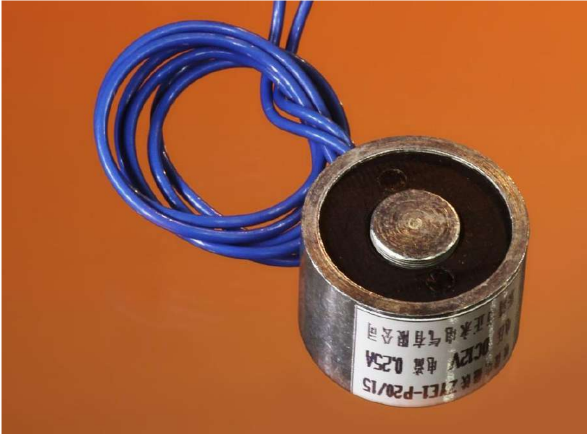
Figure 20-1. An electromagnet approximately 1 inch in diameter, rated to draw 0.25A at 12VDC.
