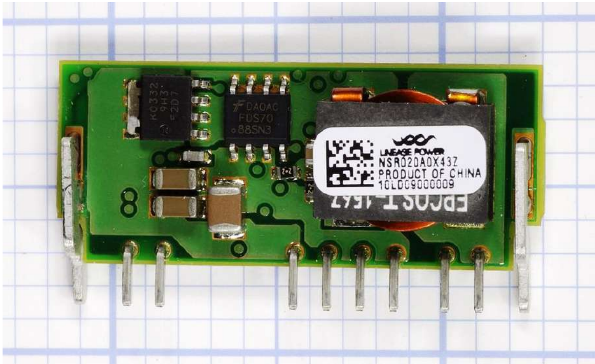
Figure 17-10. Another adjustable DC-DC converter. The output voltage is determined by adding an external resistor or trimmer potentiometer. External smoothing capacitors are required, as shown in the component's datasheet.
