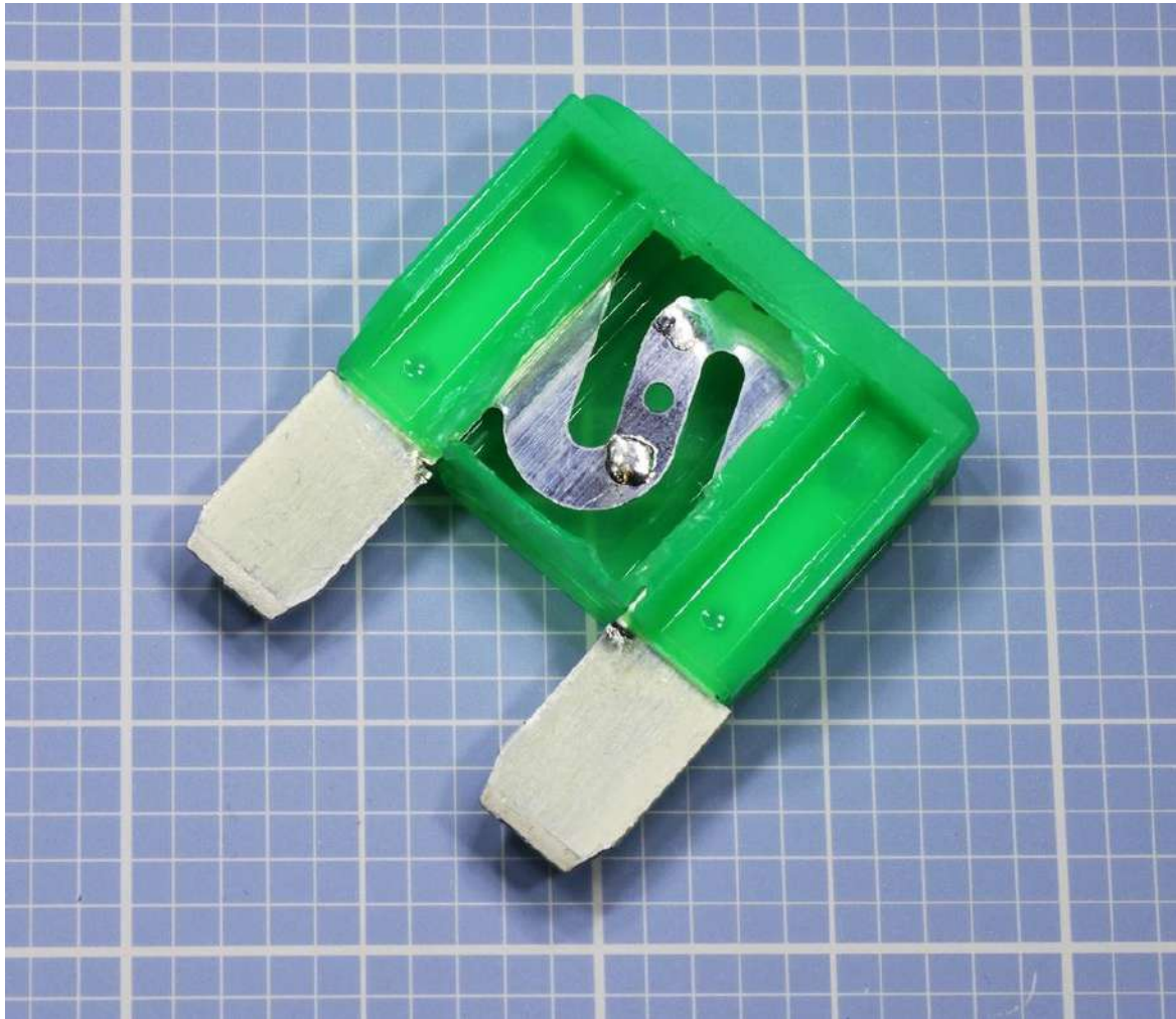
Figure 4-5. The largest fuse from the previous figure, cut open to reveal its element.
