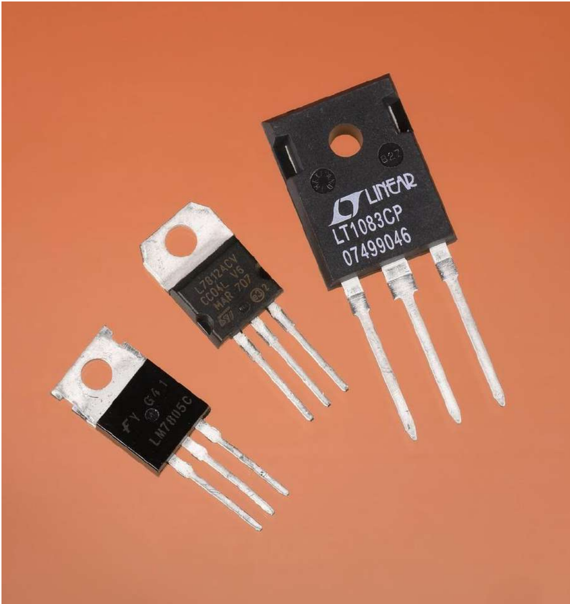
Figure 19-5. Two voltage regulators from the LM78xx series, and a third high-current, low-dropout, adjustable regulator rated 5VDC (adjustable upward) at 7.5A.
