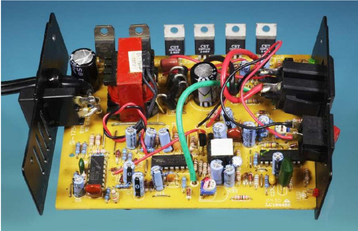
Figure 18-1. The interior components in a 175-watt inverter.
