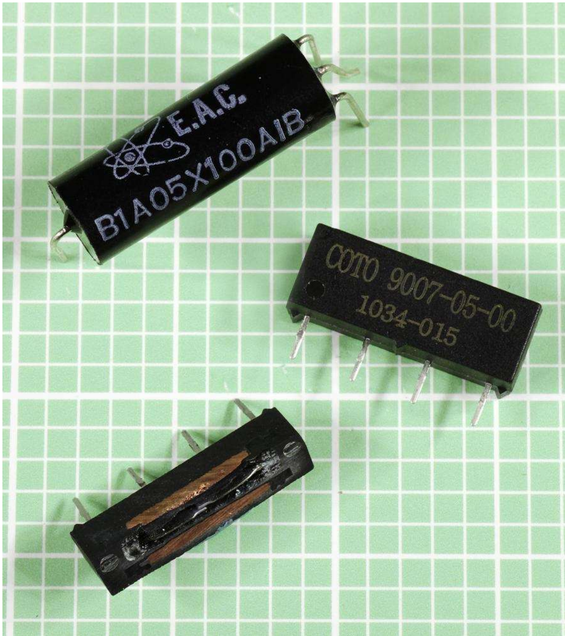
Figure 9-8. Three reed relays, one of which has had its packaging partially removed by a belt sander to reveal its copper coil and internal contacts.
