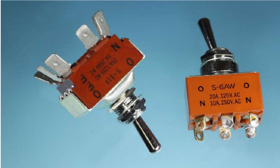
Figure 6-11. Two full-size toggle switches capable of handling significant current. At left, the switch terminates in quick-connect terminals. At right, the switch has solder terminals (some of them containing residual traces of solder).
