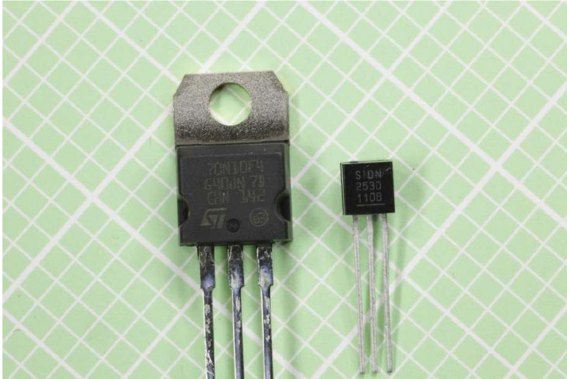
Figure 29-9. Two MOSFETs. At left, the TO-220 package claims a drain current of up to 65A continuous, and a drain-to-source breakdown voltage 100V. At right, the smaller package offers a drain current of 175mA continuous, and a drain-to-source breakdown voltage of 300V.
