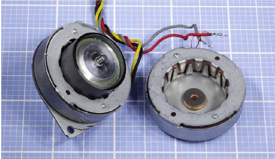
Figure 25-6. A two-deck stepper motor split open to reveal its rotor (left) and one of the stators (right) encircled by a coil.
