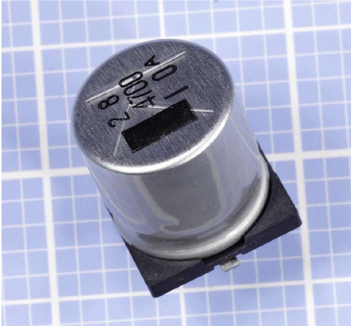
Figure 12-8. Most surface-mount capacitors are as tiny as other surface-mount components, but this 4,700 \mu F electrolytic (at 10V) has a base approximately 0.6" square. A solder tab is visible at the center of the nearest edge.
