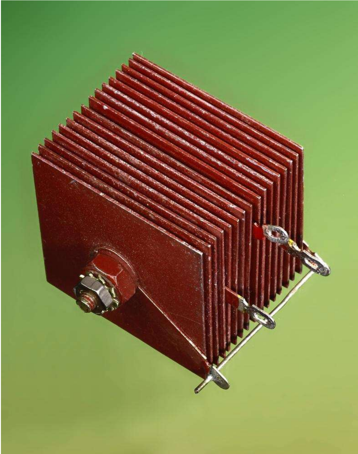
Figure 26-11. Prior to the perfection of chip fabrication in the late 1960s, it was common to find silicon rectifiers of this type, measuring about 2" square.
