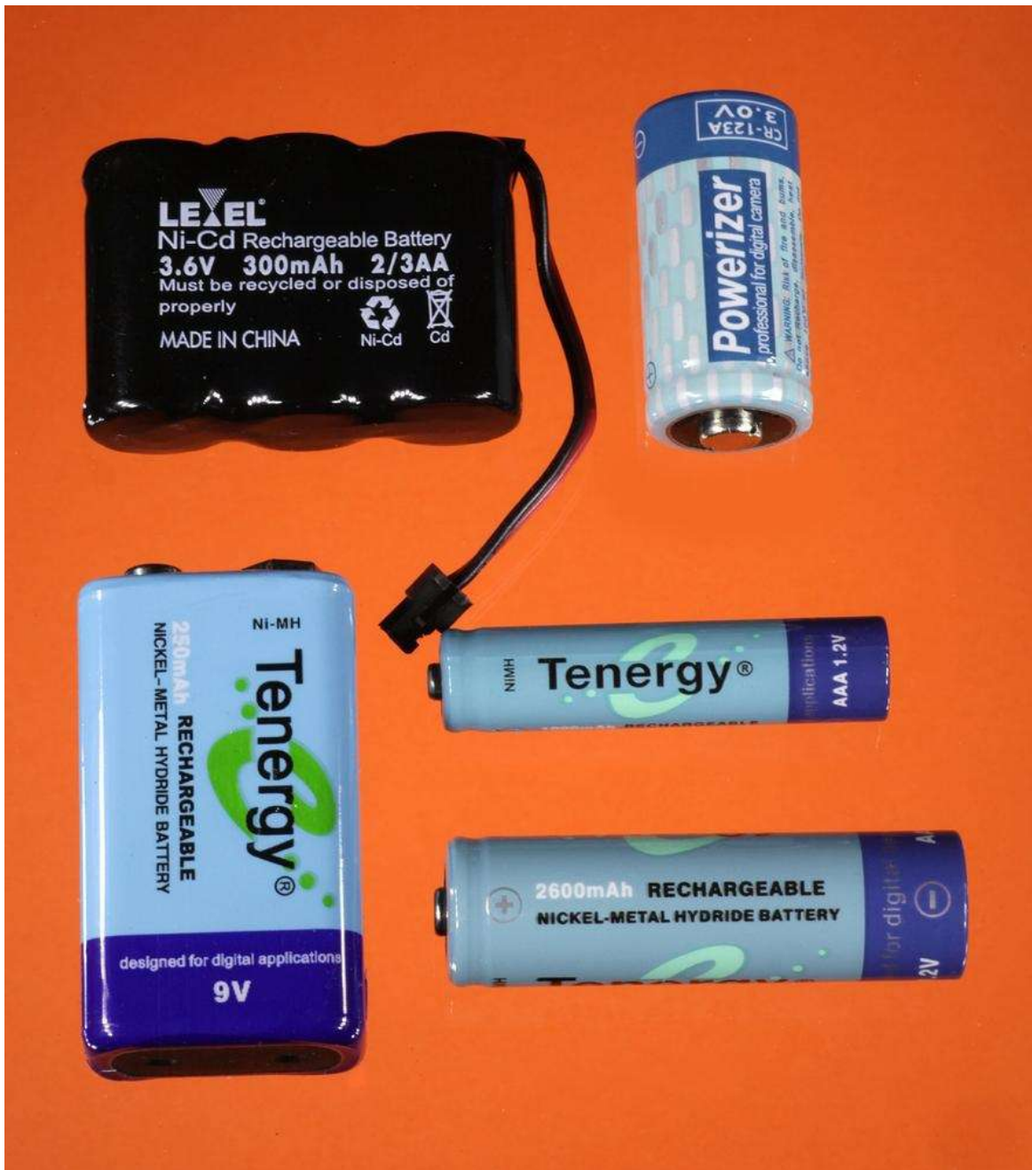
Figure 2-9. Top left: NiCad battery pack for a cordless phone. Top right: Lithium battery for a digital
