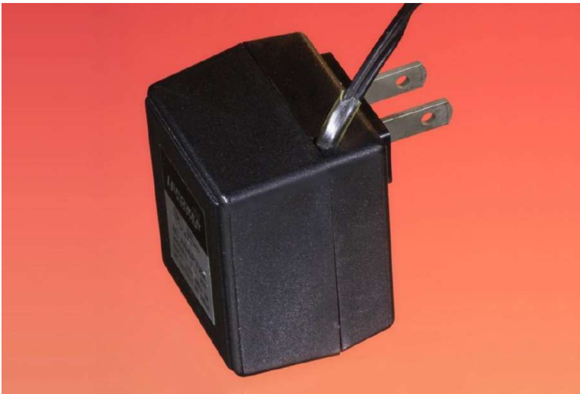
Figure 16-2. A simple transformer-based power supply can be encapsulated in a plastic shell, ready to
