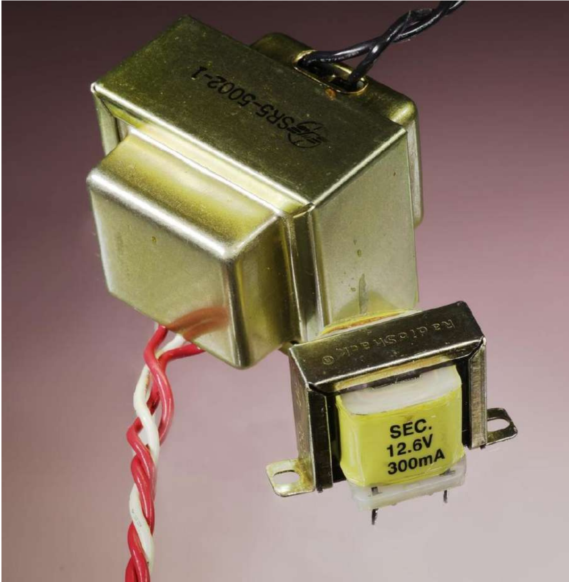
Figure 15-1. Two small power transformers. The one at the rear measures approximately 1" × 2" × 2" and is rated to provide 36VAC at 0.8A. The term "sec" on the smaller unit is an abbreviation for "secondary," referring to the rating for its secondary winding.
