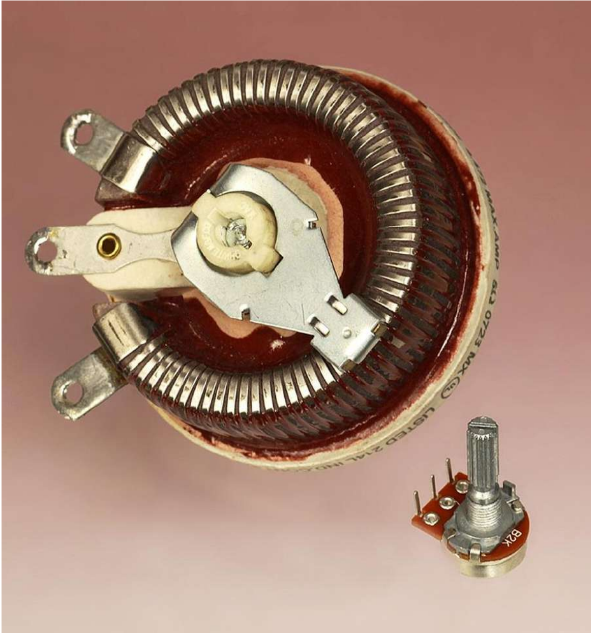
Figure 11-13. The large potentiometer is approximately 3" in diameter, rated at 5 ohms, and able to handle more than 4 amps. The small potentiometer is 5/8" diameter, rated at 2K and 1/4 watt, with pins designed for through-hole insertion in a circuit board, and a grooved shaft that accepts a push-on knob. Despite the disparity in size, the principle of operation and the basic features are identical.
