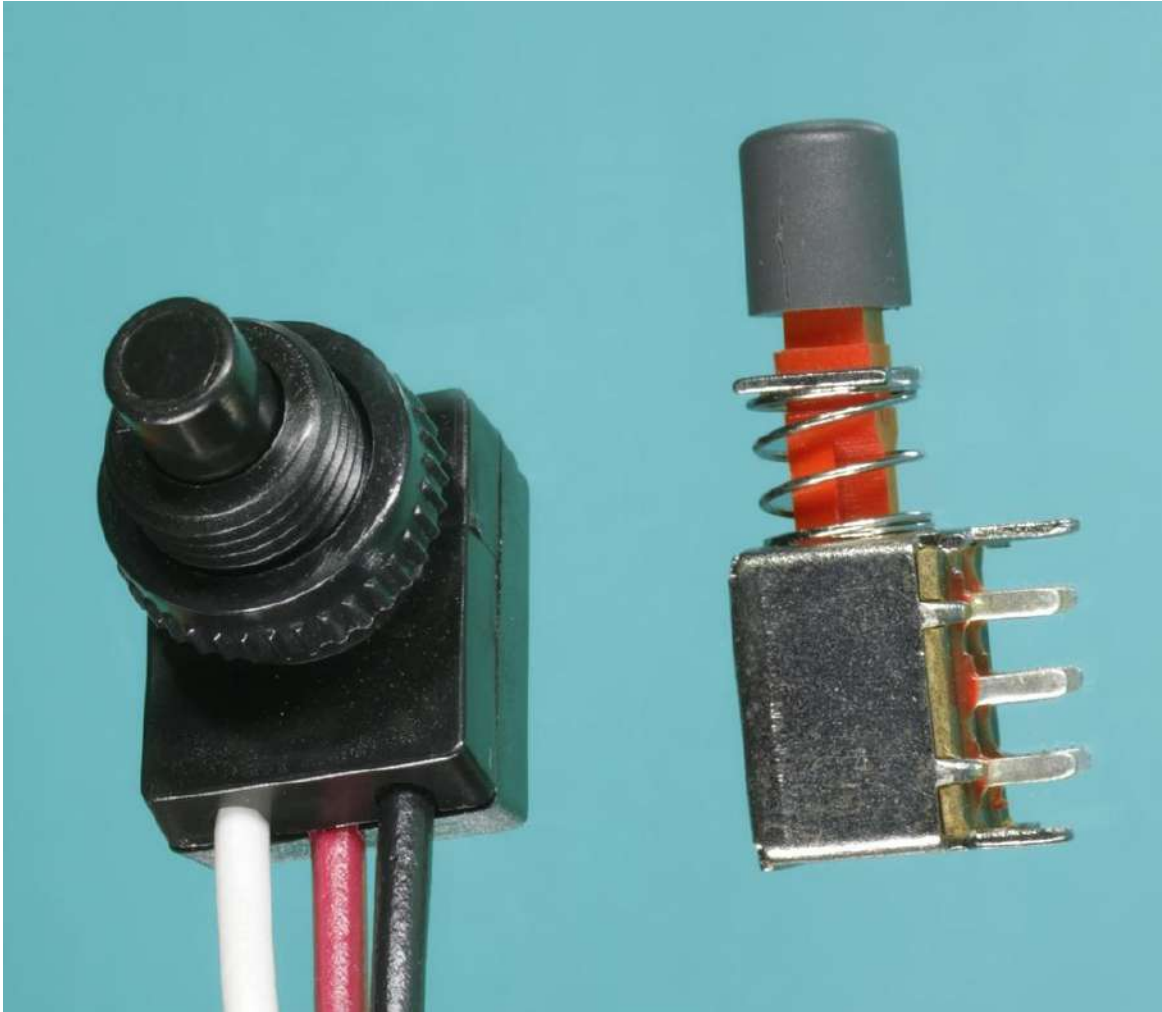
Figure 5-10. At right, a simple DPDT latching pushbutton with lockdown. At left, this pushbutton cycles through four states, one of them an "off" state, the others connecting a different pair of its wires in turn.
