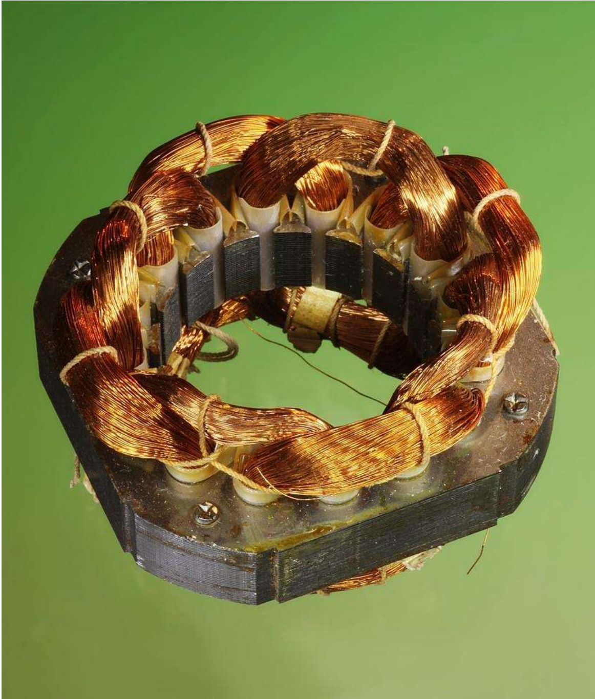
Figure 23-2. The stator from a large electric fan. Each coil of copper wire is centered on a lug pointing inward to the hole at the center, where the rotor would normally be mounted. The coils overlap because their diameter is maximized to increase their magnetic effect. Each coil is tapped to allow speed selection in steps via an external rotary switch.
