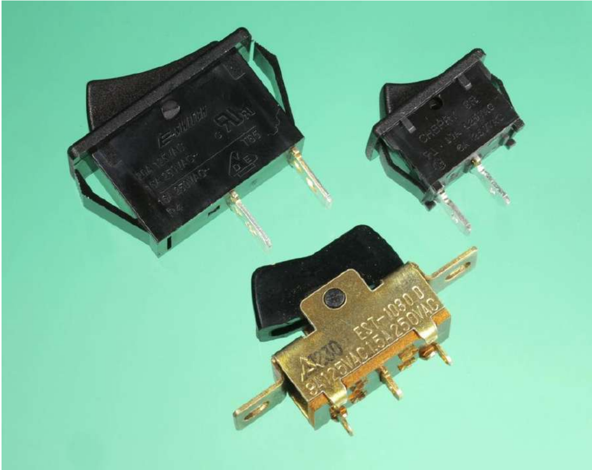
Figure 6-6. Three rocker switches, the upper two designed for push-insertion into a suitably sized rectangular hole in a panel. The switch at front-center is intended to be screwed in place, and is more than 20 years old, showing that while the choice of materials has changed, the basic design has not.
