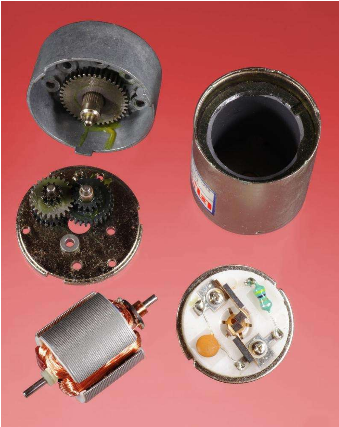
Figure 22-7. Spur gears from a gearhead motor provide speed reduction and increased torque.
