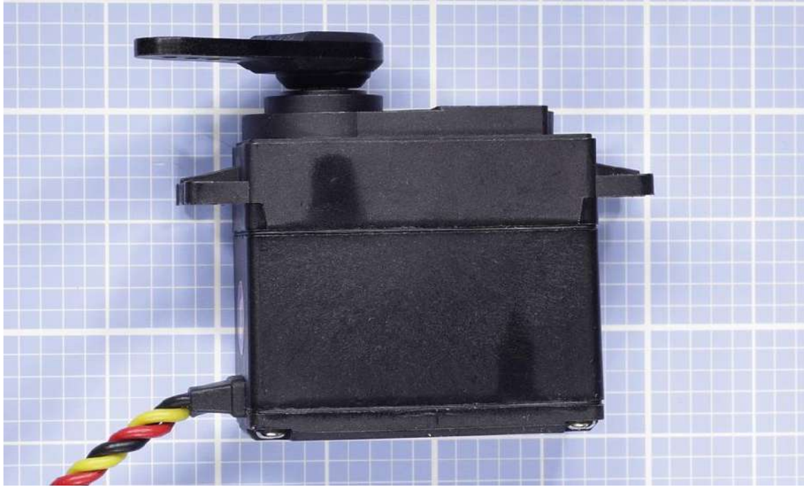
Figure 24-2. RC servo motors are mostly similar in size. This is a typical side view.
