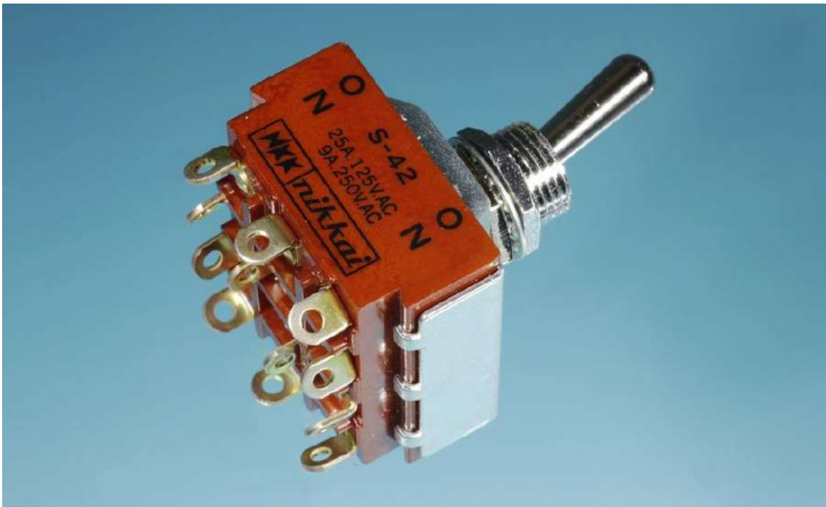
Figure 6-12. A 4PDT full-size toggle switch with solder terminals, capable of switching 25A at 125VAC. Four-pole switches are relatively unusual.
